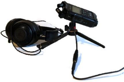
Use the splitter when you have only a microphone input on the camera. Connect the headphones to the splitter. Connect the aux cable to the second splitter input and the other end of the aux cable to the microphone port of your camera.
