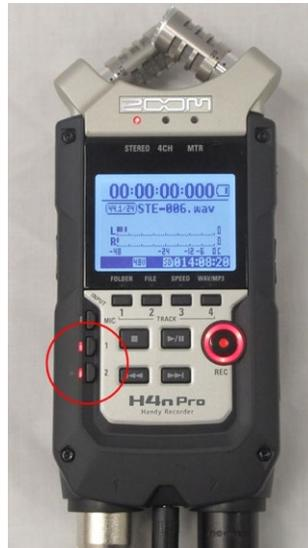
Hit REC once to enter standby mode. The ring around the REC button blinking indicates this. You will see the levels from each microphone and make adjustments before recording. To adjust have each person speak into their microphones and adjust the input volume using the REC LEVEL buttons (located on the side of the H4n under the menu button).
