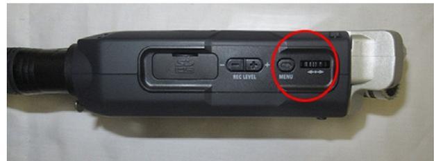
Power on (use the slider located on the left side of the H4n, slide down to power on)
